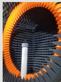
Anechoic Chamber 400 MHz - 18 GHz
